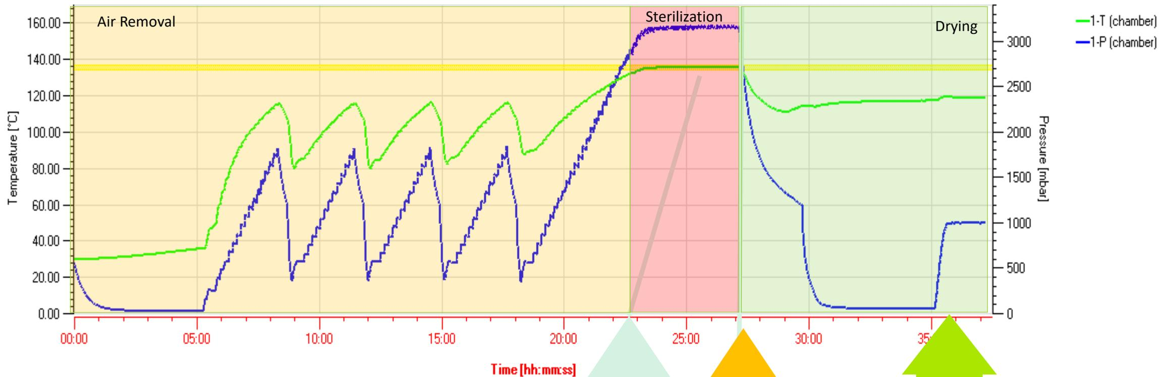
At this point sufficient air removed from all load surfaces (external and internal) to ensure presence of moisture and load at sterilizing temperature.
